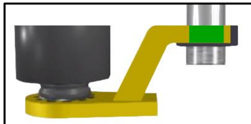
Figure 5.1.4-1: Correct Reaction Point
