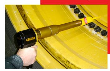
Some jobs require access to tight or hard-to-reach spaces. RAD Torque Systems offers a wide range of solutions for these common but difficult applications, including OTR wheel bolting applications. We offer nose extensions with a fixed reaction paddle, as well as ones without any reaction arm to facilitate additional flexibility.
