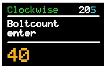
Figure 3.3.4-5: Bolt Counter Screen
