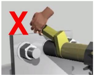
Figure 4.2.1-2: Incorrect Placement of Hand/Body Parts During Operation
