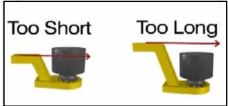
Figure 4.2.2-2: Incorrect Height IMPROPER REACTION WILL VOID WARRANTY AND CAN CAUSE PREMATURE TOOL FAILURE.
