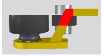
Figure 4.2.4-2: Incorrect Reaction Point
