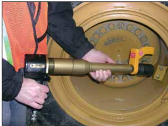
RAD 10GX (12818), 12" nose extension (14195), with reaction arm (13512)
